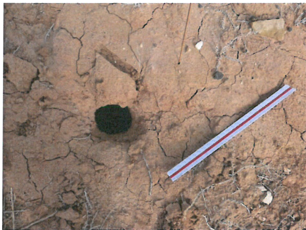
Photo D.3-15 Hole H-12 (0.4'W x 0.35'L x 1.3'D)
