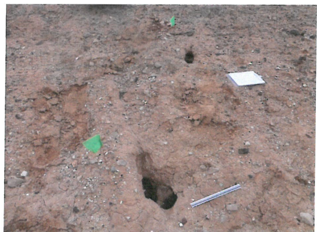
Photo D.3-6 Hole H-4 (0.8'W x 1.6'L x 2.6'D)
