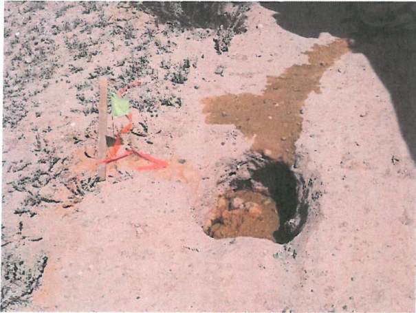
Photo D.2-A2-1 – T-5 location: Looking northeast over H-2 after presoaking and staining prior to exploration.
