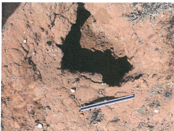
Photo D.3-47 Hole H-45 (1.8'W x 1.4'L x 1.6'D)
