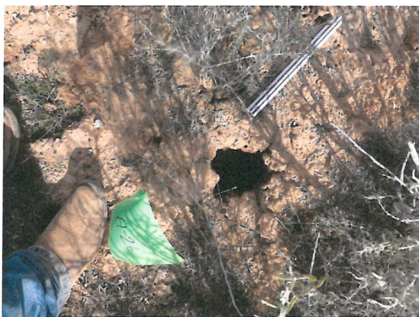
Photo D.3-29 Hole H-26(0.45'W x 0.4'L x 1.35'D)
